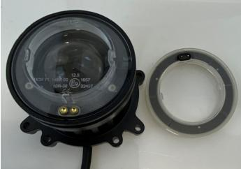
The lens have grooves in it that matches the halo so you cant put in on wrong.
