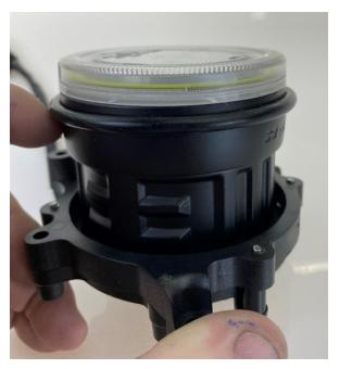
Install the light like the picture shows, use the longer torx screws and longer springs. The springs is being installed as the stock springs to create tension on the construction and to keep the possibility to adjust the lights.
