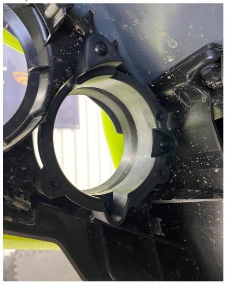
Use the OE screws with the plastic adjustment head on the high beams. NOTE put the springs on the screws before you put the lights in place this saves time and it is easier to get everything to line up.
